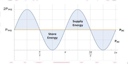
Figure 3. Instantaneous power mismatch between the DC and AC ports of a Single Phase Inverter and indication of where the energy storage device will store and supply energy.
