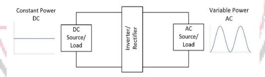
Figure 1. General arrangement of an AC to DC or DC to AC converter indicating power waveforms of the source and load.
