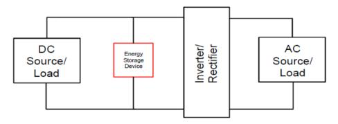
Figure 2. General Arrangement of an AC to DC or DC to AC converter with an energy storage device included.
